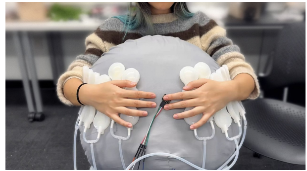
Figure 1: User interacting with Puffer by placing their finger on the pulse sensor while hugging.
